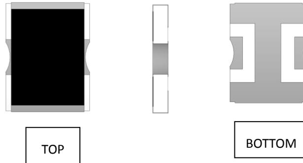
二、Effective drawing shows as below after completion of part soldering,soldering will be done with the contact of bottom side and microstrp line, black isolating resin must be upwards. It may have influence on the part reliability if not use part with correct soldering in comply with operation instruction.
