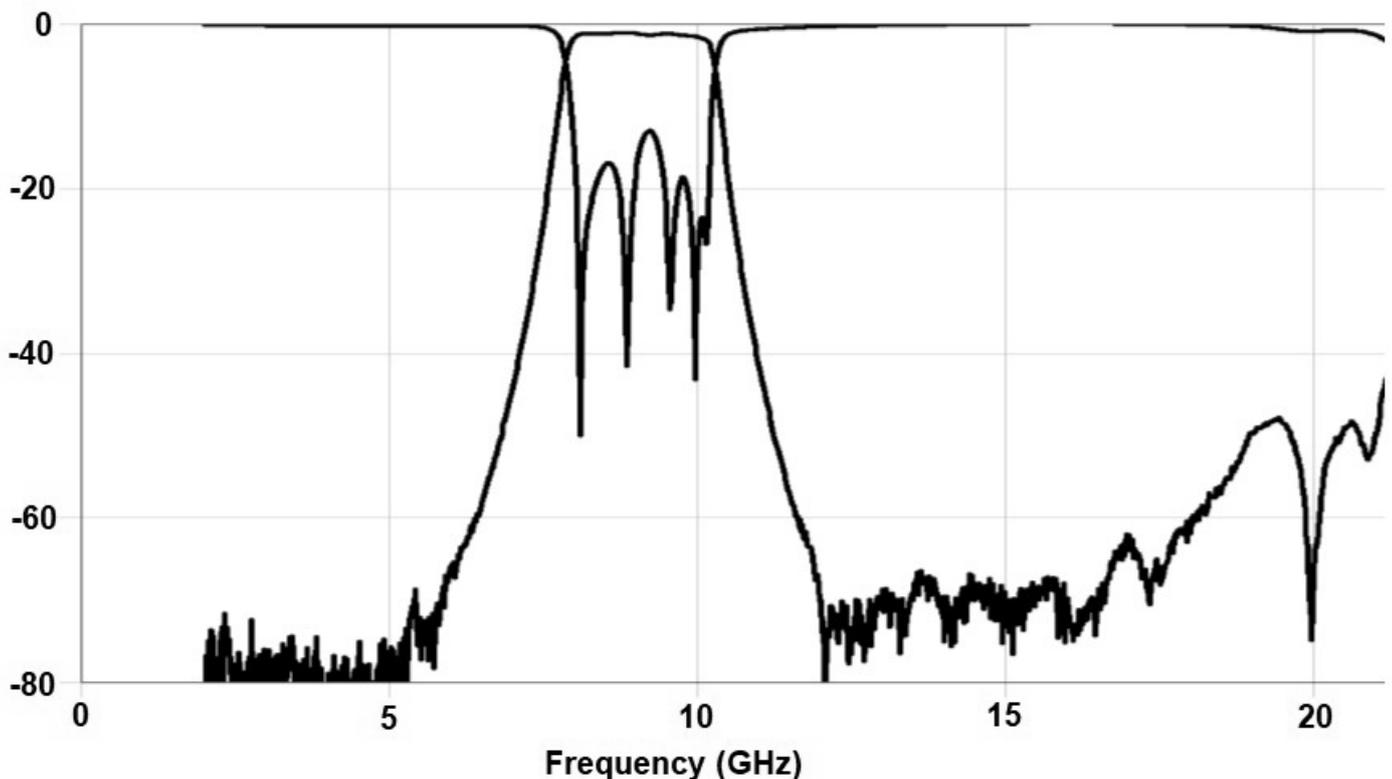
\*Typical de-embedded measured performance mounted on a connectorized test fixture. DEB is 0.254mm RO4350B with 50.00hm CPW ground traces going into the ports at room temperature.
