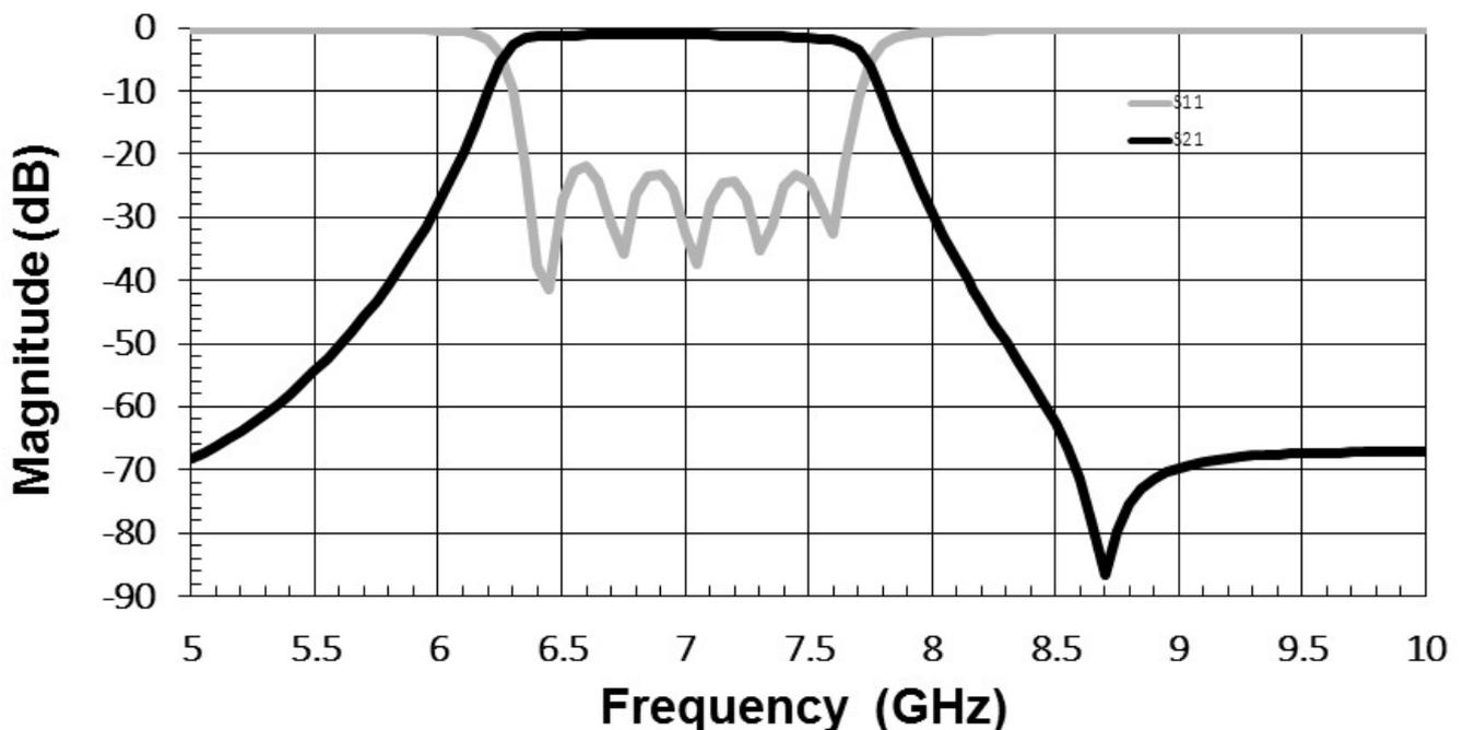
\*Typical de-embedded measured performance mounted on a connectorized test fixture. DEB is 0.254mm RO4350B with 50.00ohm CPW ground traces going into the ports at room temperature.
