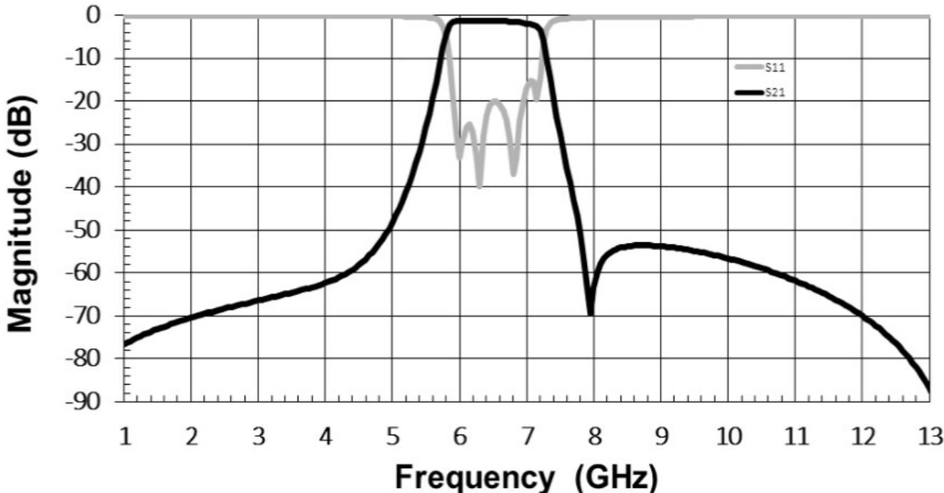
\*Typical de-embedded measured performance mounted on a connectorized test fixture. DEB is 0.254mm RO4350B with 50.0Ohm CPW ground traces going into the ports at room temperature.
