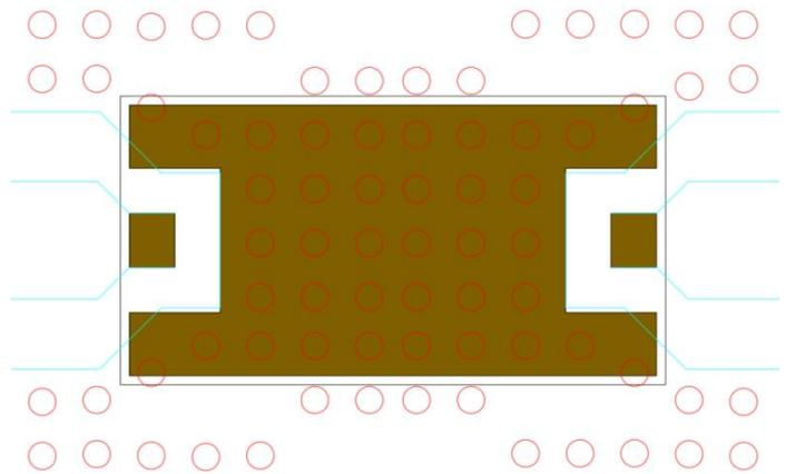
Line width to be designed to match 50 Ω characteristic impedance, depending on PCB material and thickness
