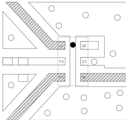
Line width to be design to match 50W characteristic impedance, depending on PCB material and thickness
